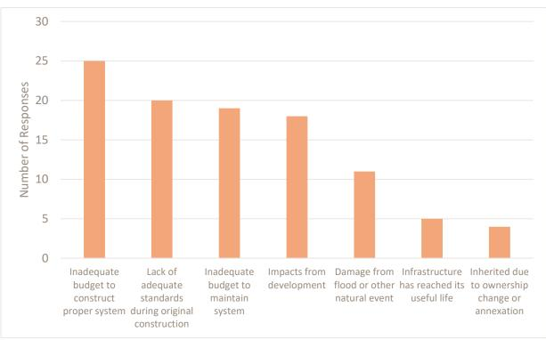
Figure 1-22: Reason for Non-Functional/Deficient Infrastructure
